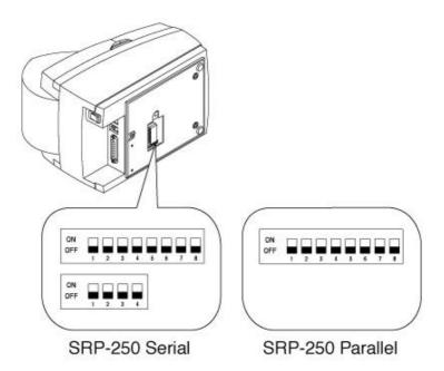
NOTE: Always change DIP switch settings when the printer is turned off. Changes made with the power on have no effect until you turn the printer off and then on again.
